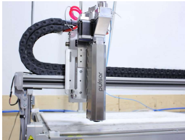
Figura 1-2: Cabezal Pulsar™ Large-Scale Pellet Extruder montado en maquina - DYZE DESIGN. (2020). PULSAR™ LARGE-SCALE PELLET EXTRUDER. 2021, DE DYZE DESIGN RECUPERADO DE HTTPS://DYZEDESIGN.COM/PULSAR-PELLET-EXTRUDER/?Gclid=CJWKCAJWQVYFBHB7EiWAER786BBc2M0RU5cBEK5vsHXTN54OGR9EBGKFIV5A8RZQEHV-kCSXKYMROXOCNU4QAVD_BWE#PLASTICS-STANDARD
