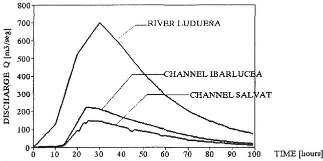
Fig. 5 Upstream hydrograph; return period 500 years, with works.
