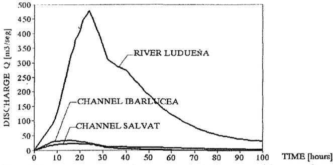
Fig. 4 Upstream hydrograph; return period 50 years, without works.
