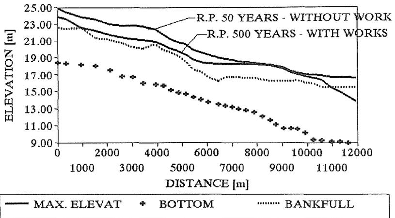
Fig. 8 Maximum elevations over river.
