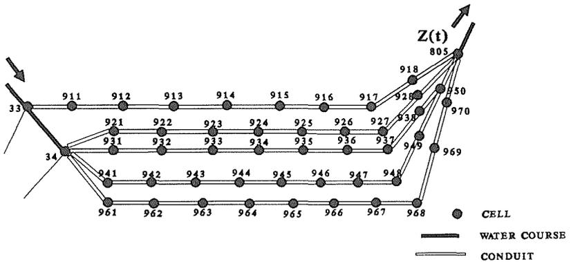
Fig. 3 Topological representation of conduit network.
