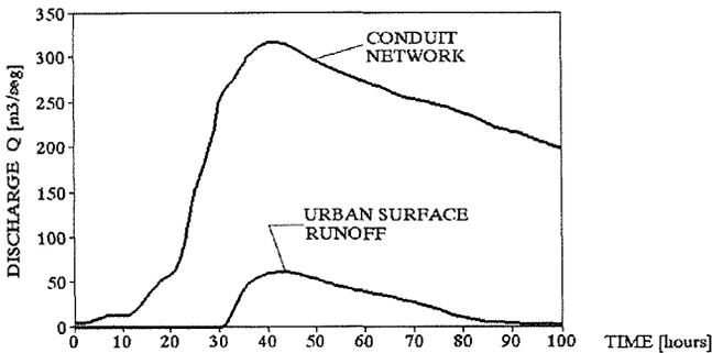
Fig. 7 Downstream hydrograph; return period 500 years, with works.
