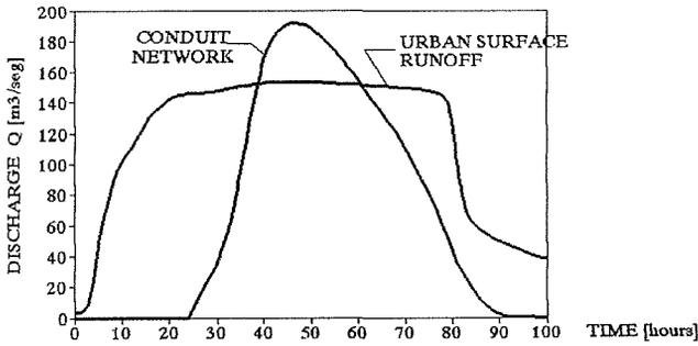
Fig. 6 Downstream hydrograph; return period 50 years, without works.
