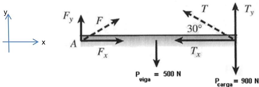
$$(1) \quad \Sigma \bar{F}_x = \bar{0} \quad \Rightarrow \quad F_x - T_x = 0$$
