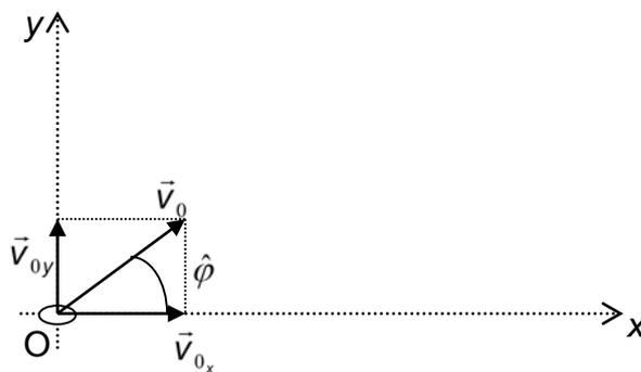
$$\left. \begin{aligned} v_{0x} &= v_0 \cdot \cos \hat{\phi} \\ v_{0y} &= v_0 \cdot \sin \hat{\phi} \end{aligned} \right\} \text{son las componentes de la velocidad inicial}$$
