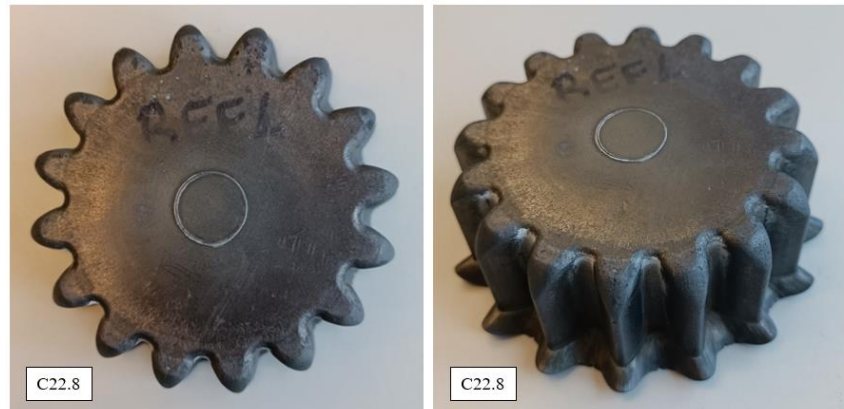
Figura 4.8: Probeta Ref. 1 de material único C22.8
