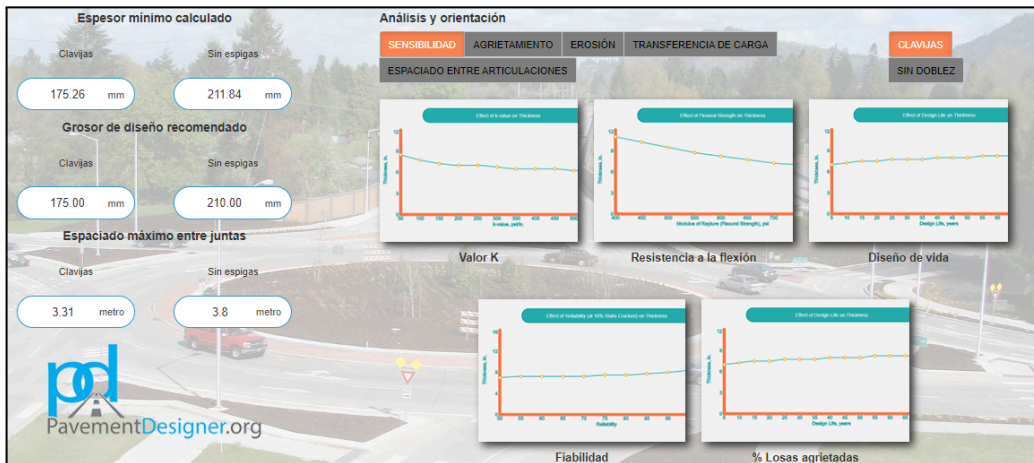
Figura 6.1.3.4. Pavement Designer Resumen general. Fuente: Pavement Designer.
