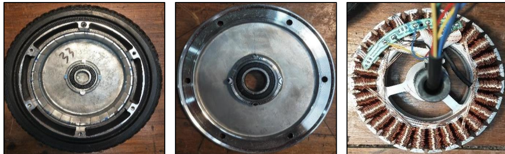
Figura 4-12: Motor PMSM in-wheel.
