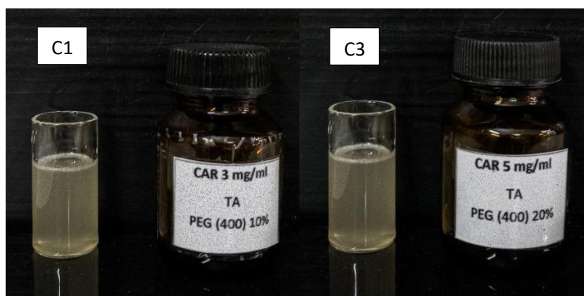
Figura 3.1.2. Control visual gotas de Carvedilol 3mg mL -1 , 10% v/v PEG 400 (C1); 5mg mL -1 , 20% v/v PEG 400 (C3)
