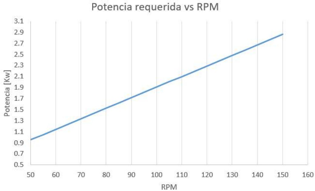
Figura 4-7: Potencia requerida vs RPM.
