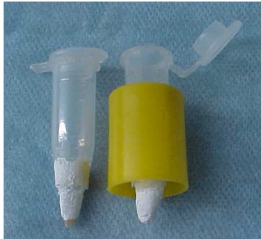
Fig. 1 Root fitted on the Eppendorf tube and it adapted into a test tube lid.
