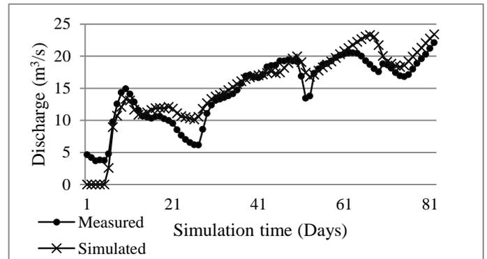
Figure 5. Measured and simulated discharges for medium flow event in gauge station No. 421147.
