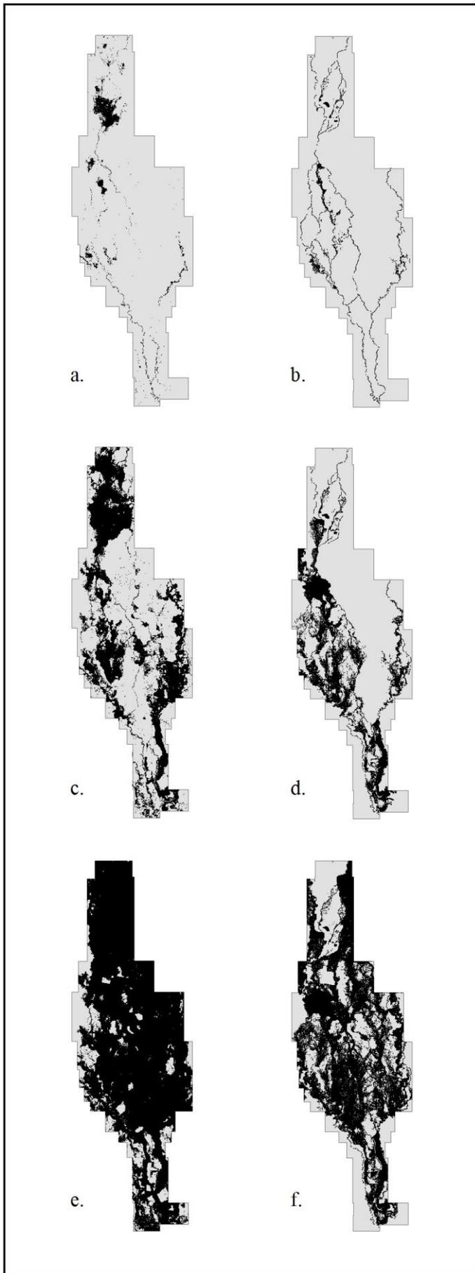
Figure 4. Inundation maps of the selected events. Remote sensing maps a, c and e for low, medium and high flow events respectively. Modeled event maps b, d and f for low, medium and high flow respectively.
