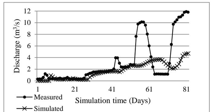
Figure 6. Measured and simulated discharges for medium flow event in gauge station No. 421152.
