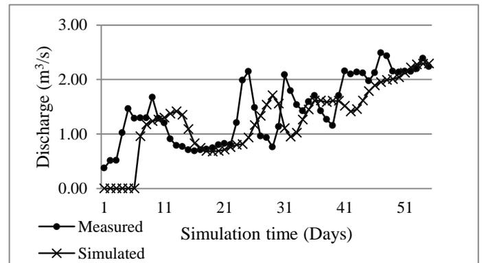
Figure 3. Measured and simulated discharges for low flow event in gauge station No. 421152.
