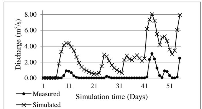
Figure 2. Registered and simulated discharges for low flow event in gauge station No. 421129.
